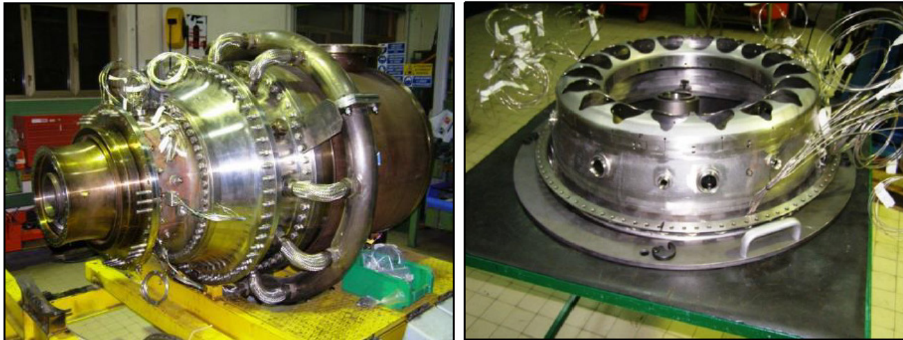
PERM Development at GE AVIO (lhs: combustor assembly; rhs: instrumented liner)
